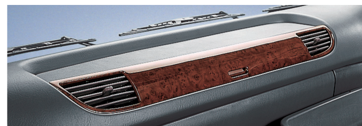
103 Wood-like Panel Relay Lid Panel (RHD) P/N:1-8671-1081-2 Installation Time:0.4H
