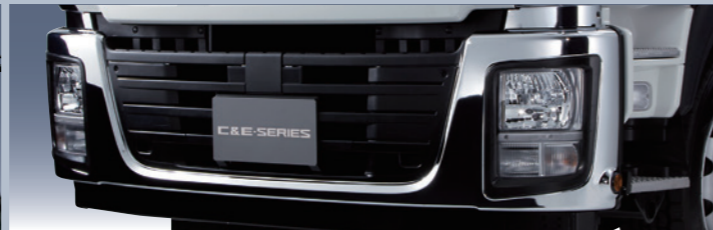
69 Chromed Front Bumper P/N:1-8671-2127-0 Installation Time:1.0H Weight:32kg
