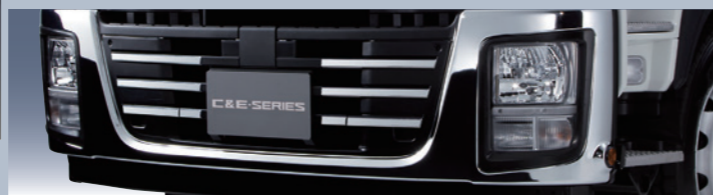
72 Chromed Bumper Grille Molding P/N:1-8671-2114-0 Installation Time:0.5H
