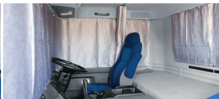
89 Round Curtain P/N:1-8671-3036-4 Installation Time:0.8H Weight:1.5kg *Round Curtain Rail Kit is required for round area. ●Round Curtain Rail Kit P/N:1-8671-3044-0 Installation Time:0.8H
