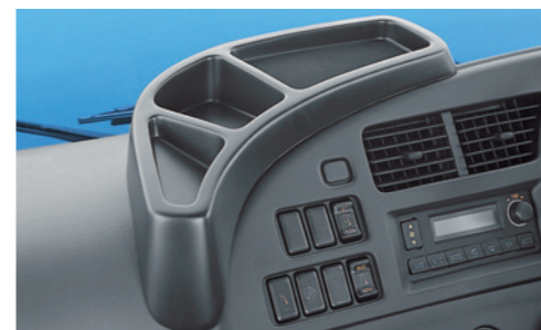
108 Instrument Panel Tray (RHD) P/N:1-8843-4464-1 Installation Time:0.3H
