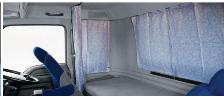
91 Bed Room Curtain P/N:1-8671-3039-3 Installation Time:0.6H Weight:0.9kg 92 Bed Room Curtain Complete Shield-type P/N:1-8671-3053-1 Installation Time:0.6H Weight:0.9kg
