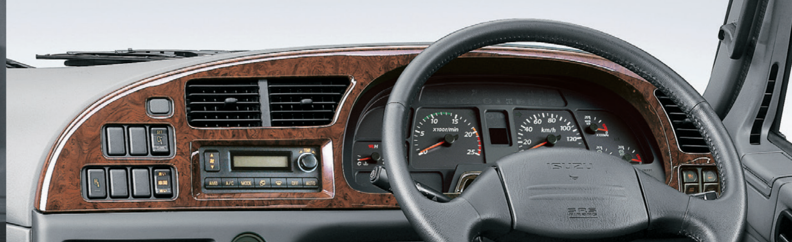
99 Wood-like Panel Meter Cluster (RHD) P/N:1-8843-4775-2 Installation Time:0.3H Material:Resin(ABS) *Installed as standard on custom vehicles.
