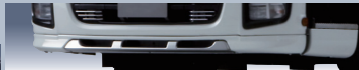
71 Front Lip Spoiler P/N:1-8671-1164-0 Installation Time:1.0H Weight:2.2kg *Cannot be installed on low-bed three/four-axle trucks with leaf spring suspensions. *Additional parts required when installing on vehicle equipped with standard bumper without air dam.
